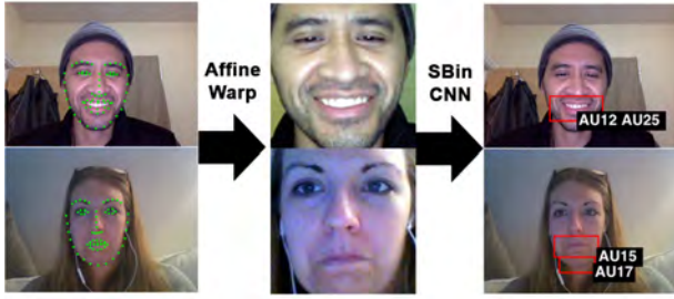
Figure 2: The face is first processed through a CLM [1] keypoint detection algorithm, then the cropped face area is affine warped to a base face shape and processed by the SBinCNN [8] algorithm to produce the AU activations.
